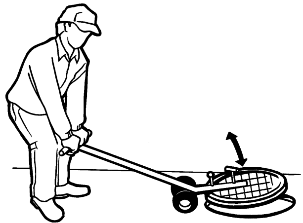
FIGURE 2 - Use levers to reduce the force required
