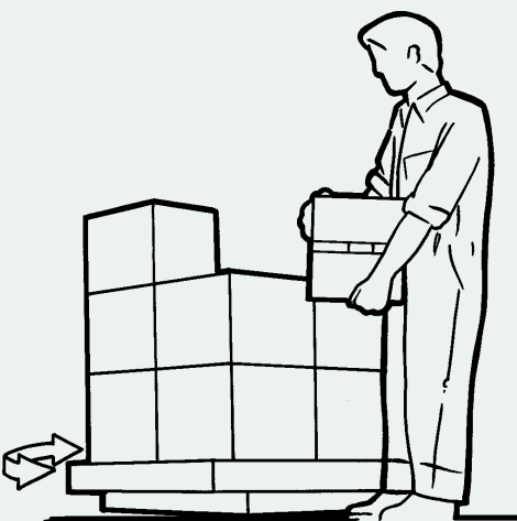
FIGURE 3 - Reducing twisting by using a pallet turntable
