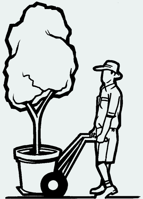
Large wheels require less force
