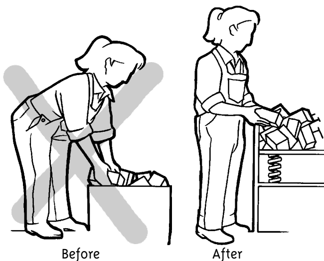
FIGURE 3 - Raise work level by use of self-adjusting platform
